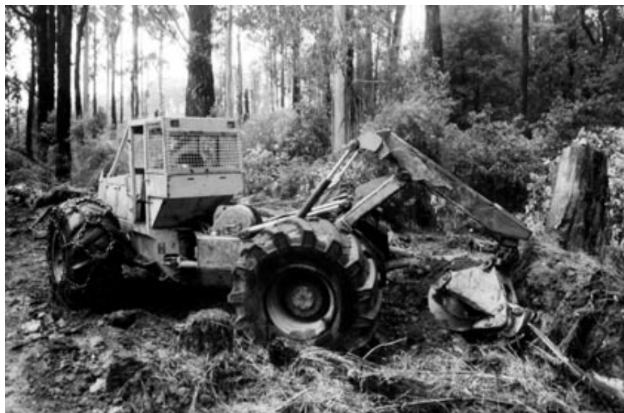
A “skidder” used to drag logs to the log landing, the Otways. PHOTO: TONY QUOLL, 1999
